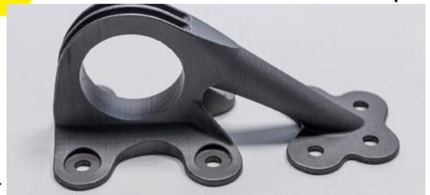
The prototype of a bracket created with 3D printers using laser melting technology caused quite a stir. This connecting element for aircraft used to be milled from aluminium.
